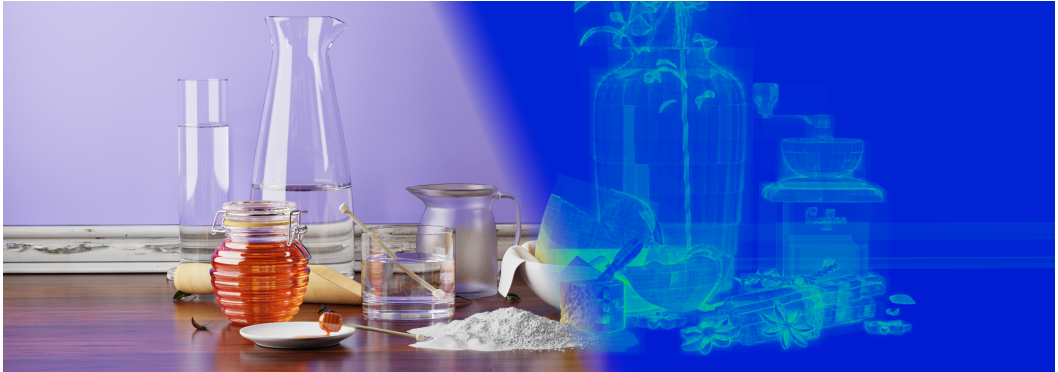
Fig. 1. Visualization of BVHs constructed with H-PLOC in Nexus Renderer [3] for the Cannelle & Fromage scene, built in a few milliseconds. Color intensity represents the number of ray-node intersections (right).
